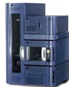
In the optional sample organizer, a ½-inch lead screw and anti-backlash nut is employed to produce the Z axis motion, allowing the robotic machine to shuttle as many as 21 sample plates back and forth to the sample manager.
