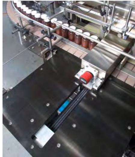
The length and speed of the Kerk RGS is not limited by critical screw speed, allowing high RPM and linear speeds, even over long spans. Standard leads include .100", .200", .500" and 1.00" travel per revolution. With Kerk’s wide range of available leads, speeds over 60 inches per second (1.5 meters per second) are possible, rivaling belts and cables while offering superior positioning accuracy, repeatability and axial stiffness.
