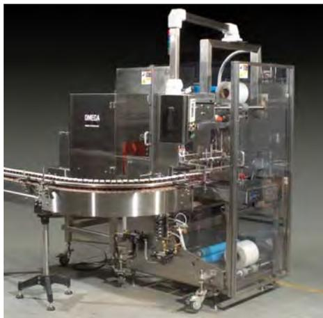
pneumatically-driven, PLC-controlled machine was designed for automatic shrink or stretch packaging of glass, plastic or metal containers, boxes or cartons into pre-determined bundle configurations. The design of the “Classic” series helps to eliminate the high cost of cardboard boxes and creates a more efficient, secure package, which lends itself to further
