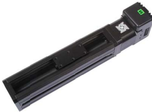
Figure 3 This assembly includes the lead screw and nut, along with guide features, motor and drive. The guide system is also a structural aluminum rail.
