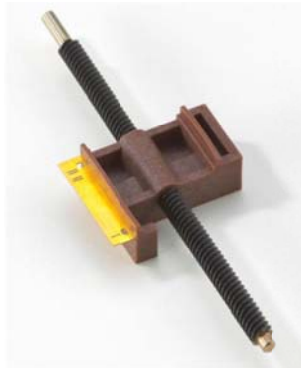
Figure 1 This self-lubricating, custom molded nut includes an insert-molded encoder strip and special guidance features. The lead screw has a low friction, PTFE lubricant coating.
