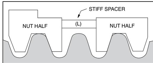
This is fine initially. However, as use time increases, wear begins on the nut threads causing a gap to develop between the spacer (L) and the nut halves.
