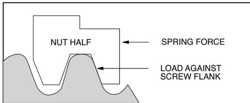
For example, if the maximum axial load to which the system is subjected is 50 lbs., the amount of spring preload must be equal to, or greater than, 50 lbs. in order to maintain intimate screw/nut contact. The problems arising from preloading in this manner are increased drag torque and nut wear.
