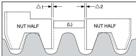
This gap ( $\Delta 1 + \Delta 2$ ) is now the amount of backlash which has developed in the unit. This backlash can be removed by replacing the stiff spacer with a new spacer equal to  $(L + \Delta 1 + \Delta 2)$ . This process, although effective, would be extremely costly and difficult to implement on a continuous basis.
